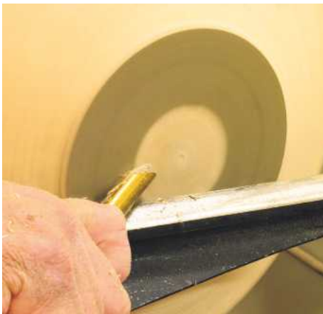
▲ Pic.4 A finer cut can be achieved by closing the flute and turning the cut into more of a shear cut. Les is using it just to true up the base
